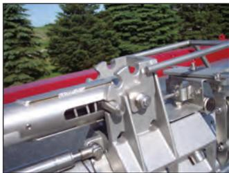
The TRAM arm has a 3-position lock mechanism. The arm is stored horizontally when not in use. The arm also locks at 45° or vertical, providing two working heights.
