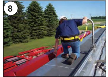
8 The harness straps give the operator adequate flexibility when performing tasks.
