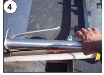
4 The arm is unlocked and raises to 45° or vertical position. A gas strut keeps movement predictable and steady.
