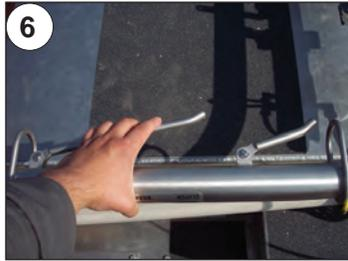
6 Pulling the TRAM brake lever releases the arm and allows it to slide on the rail. Releasing the brake lever locks the arm in place on the rail.
