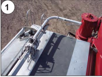
1 The TRAM arm in transport position. The position of the arm aids operator access from the rear body platform.
