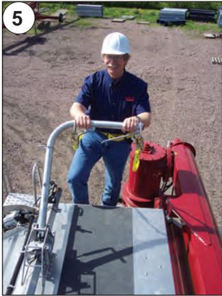
5 The TRAM arm is raised and locks itself in place. The gas strut actually assists the operator in getting up on the trailer.
